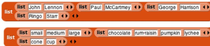
We can also build any classic computer science data structure out of lists of lists, by defining *constructors* (blocks to make an example of the structure), *selectors* (blocks to pull out a piece of the structure), and *mutators* (blocks to change the contents of the structure) as needed. Here we create binary trees with selectors that check for input of the correct data type; only one selector is shown but the ones for left and right children are analogous.
